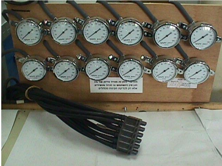
A. 12 pressure gauges board and hose bundle
